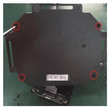
2.4 Install the base side cover and fixed 4 M2\*5 screws.
