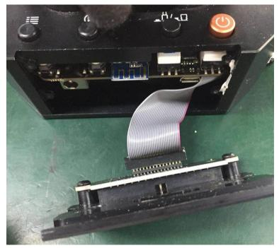
1.3 Remove 4 M3\*5 screws on the bottom of the uArm base bottom cover.
