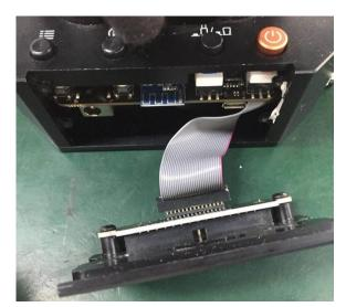
3. Remove 4 M3\*5 screws on the bottom of the uArm base
